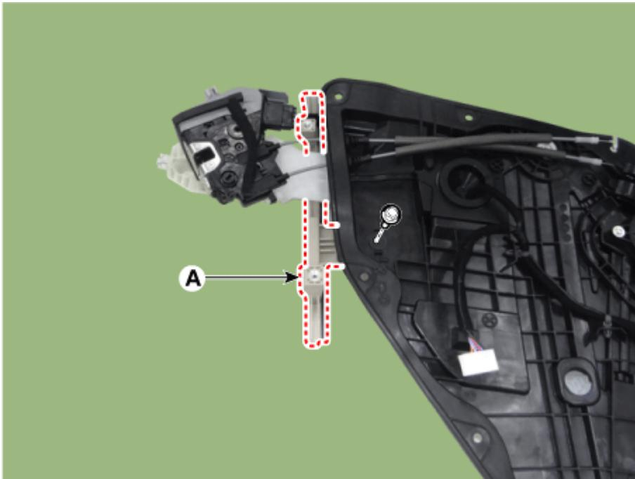
10. Remove the rear door latch (B) after disconnecting the latch connector (A).
