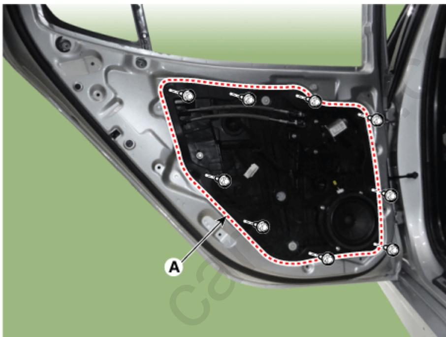
9. Remove the rear door channel (A) after loosening the mounting bolts.
